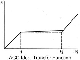
For low input signals the AGC is disabled and the output is a linear function of the input, when the output reaches a threshold value (V1) the AGC becomes operative and maintains a constant output level until it reaches a second threshold value (V2). At this point, the AGC becomes inoperative again; this is usually done in order to prevent stability problems at high levels of gain.
