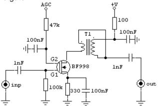
Dual-gate MOSFET amplifier controlled by AGC
