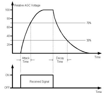
Relationship between signal level and Attack and Decay characteristics of an AGC system
