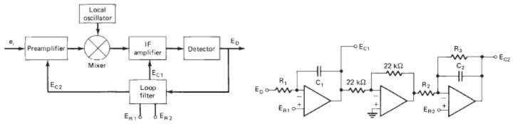
On the other hand, reduction of the preamplifier gain increases the NF of the system. Low NF is the reason for using the preamplifier stage in the first place. To solve these difficulties, it is necessary to delay application of AGC to the preamplifier until the gain in the later stages has been sufficiently reduced by the input level.
